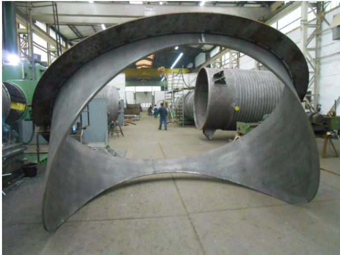
Manufacturing and mounting (Netherlands) Sea water condenser Ø 3.650 mm, overall length 10.000 mm, 40 t, 1.4462/P355GH
