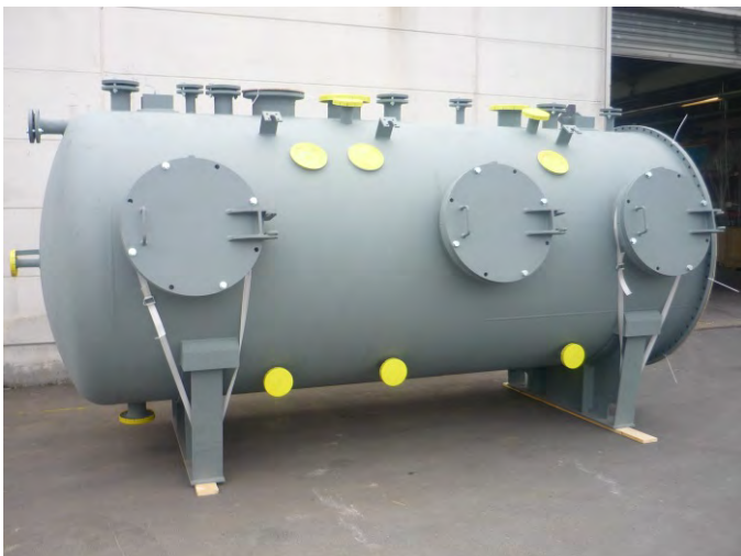
Crystallizer part Ø 1.800 mm, steel/rubber lined
