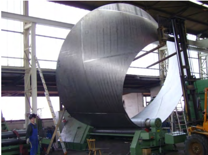
Site fabrication and mounting (Austria) Evaporation crystallizer \varnothing 6.400 mm, overall length 18.700 mm, 56 t, 1.4562
