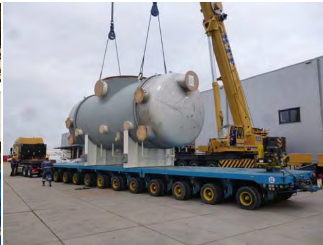
Manufacturing and mounting (Netherlands) Sea water condenser Ø 3.650 mm, overall length 10.000 mm, 40 t, 1.4462/P355GH
