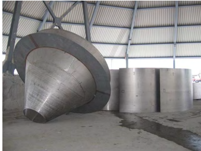
Site fabrication and mounting (Austria) Evaporation crystallizer \varnothing 6.400 mm, overall length 18.700 mm, 56 t, 1.4562
