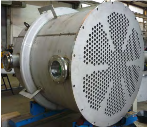
Oleum condensator Ø 1.650 mm, 1.4571
