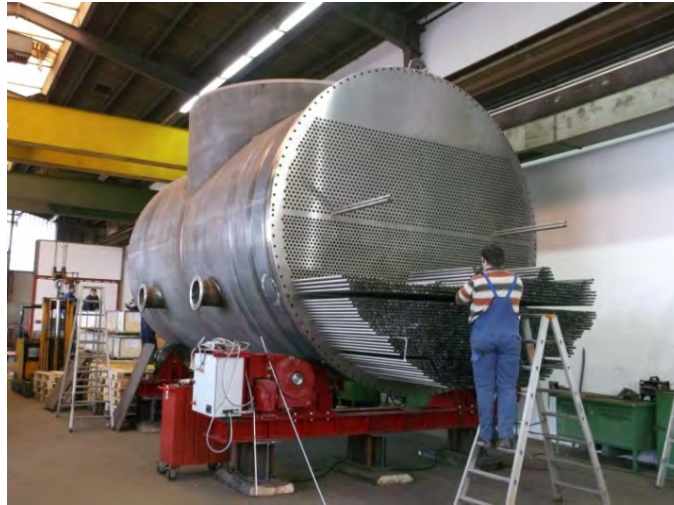
Manufacturing and mounting (Netherlands) Sea water condenser Ø 3.650 mm, overall length 10.000 mm, 40 t, 1.4462/P355GH
