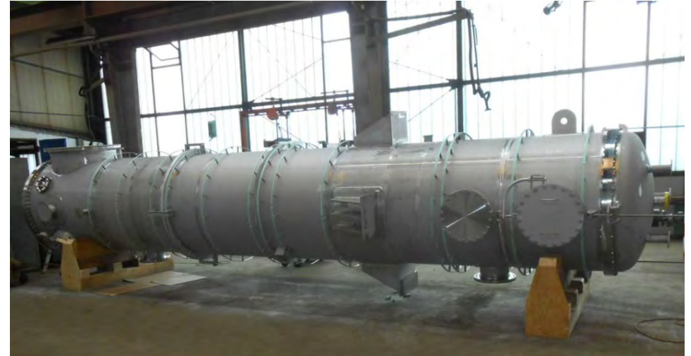
Plume-condensator Ø 1.800 mm, 1.4541
