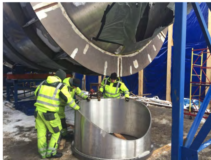
Site fabrication and mounting (Russia) Evaporating crystallizer Ø 5.400 mm, overall length 21.800 mm, 40 t, 1.4562
