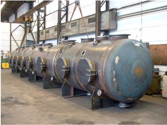
Flash evaporator Ø 3.500 mm, steel/rubber lined
