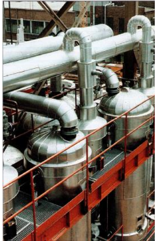
Crystallization plant for glauber's salt with NH 3 -cooling/芒硝结晶
