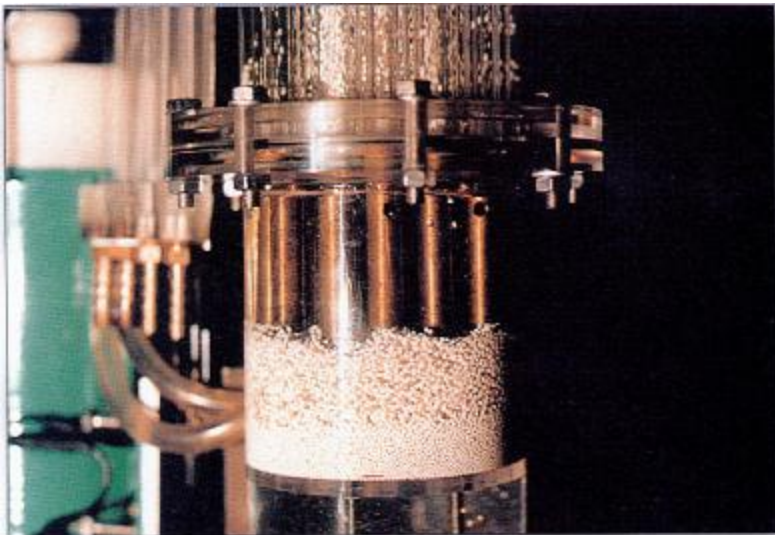
Solid particles in the inlet chamber of the fluidized bed heat exchanger/ 流化床换热器列管中的固体颗粒
